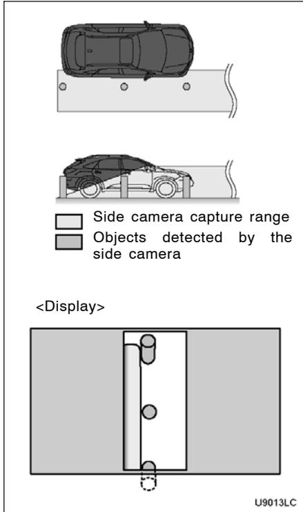
● When a 3-dimensional object is near the vehicle
