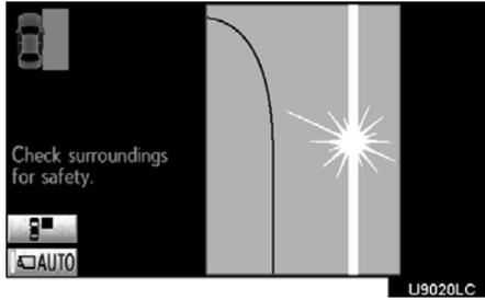
If a bright light (for example, sunlight reflected off the vehicle body) is picked up by the side camera, the smear effect\* peculiar to CCD cameras may occur.
