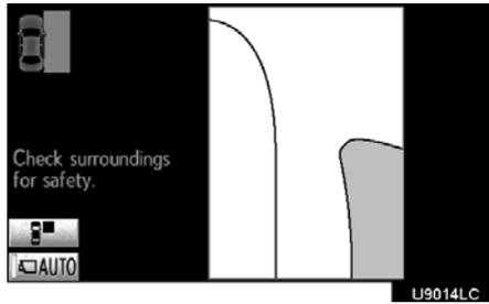
On the display, it appears that the vehicle will not hit the wall. In reality, the overhanging part of the wall is in the way, and the vehicle may collide with it. When the course is close to an obstacle, be sure to check the vehicle's surroundings with your own eyes and the vehicle's mirrors.
