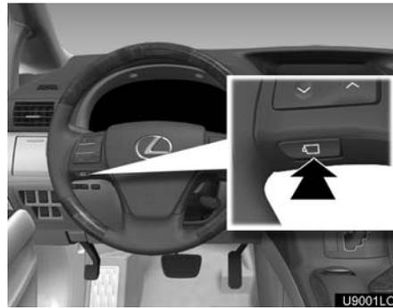
To display the side view, push the side camera button with the “ENGINE START STOP” switch in **ACCESSORY** or **IGNITION ON** mode and vehicle speed at **7 mph (12 km/h) or less**.
